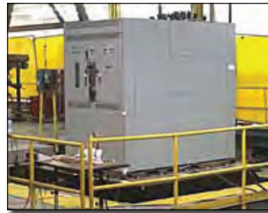
This stop-action image shows a 4000 amp bypass-isolation automatic transfer switch withstanding thousands of pounds of force in three directions. The enclosure can move as much as three or four inches. Photo: Courtesy of ASCO Power Technologies
