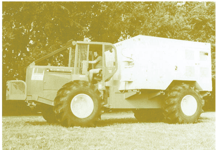
This all-terrain vehicle carries a 2-ton payload of sensitive geophysical instruments and self-contained power supply in a "doghouse" isolated from the chassis on twelve Aeroflex mounts.
