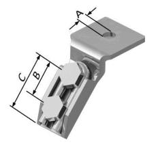
**Installation:** Use SB-125's with standard 1-5/8" strut, ASTM A-307 Grade A bolt, and standard washer when directly attaching to building structure.
