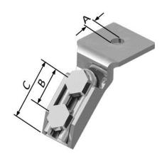
**Installation:** Use SB-250's with standard 3 x 2 x 3/16" angle, ASTM A-307 Grade A bolt, and standard washer when directly attaching to building structure.
